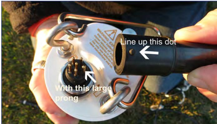
6. Push the cable plug over the pins and then screw on the plug cover.
