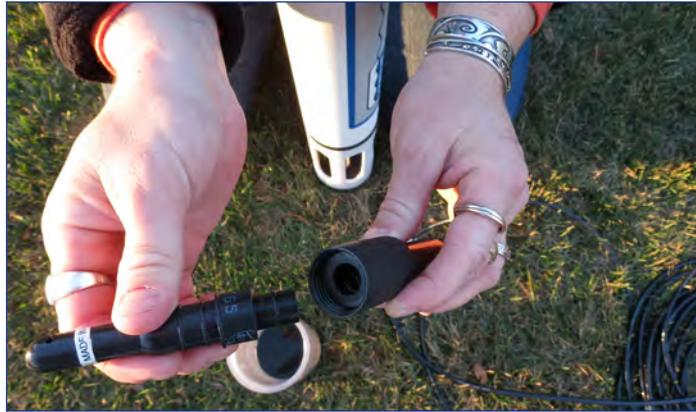
2. Line up the raised dot on the cable with the large prong. Be careful with the pins!
