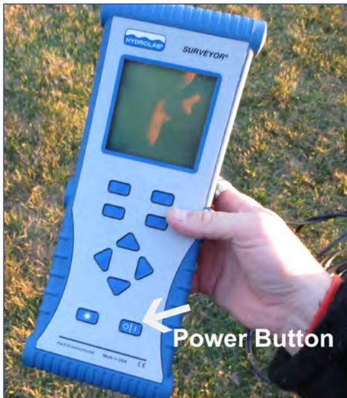
12. Find the barometric pressure on the Surveyor screen. It will say *BP*. (If it is not on the display, refer to *Setting up the Surveyor Display* on page 11.) You will need this number to calibrate the DO%.
