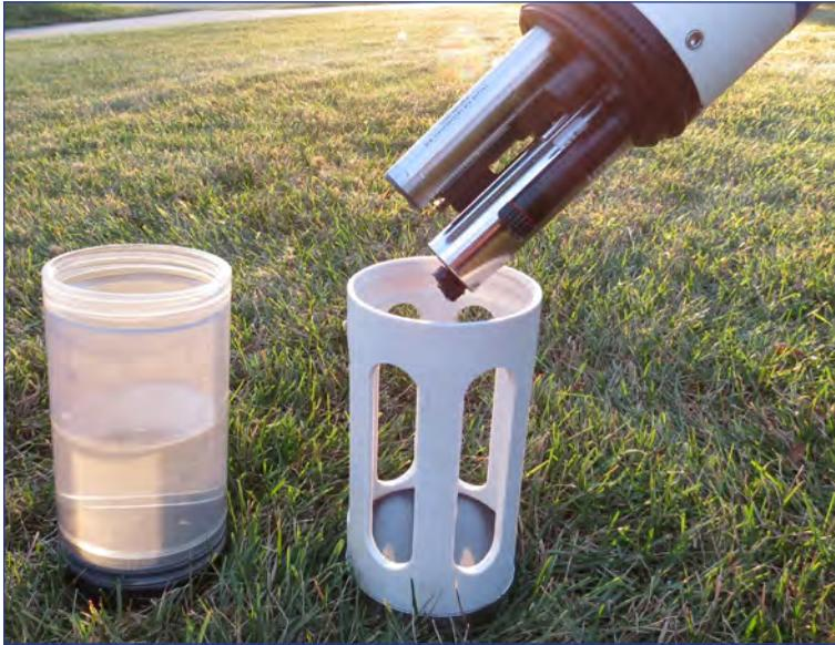
2. Remove the sensor guard from the Hydrolab and screw on the calibration cup.
