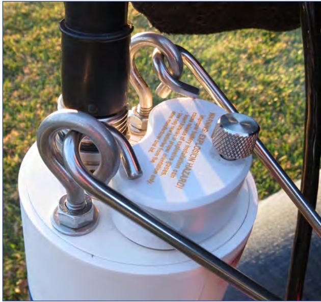
4. Attach the deploying line to the Hydrolab using the screw link.
