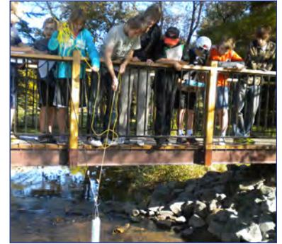
There are several characteristics of water that can be measured to assess water quality. Each Hydrolab DS5 DataSonde contains sensors that measure seven standard parameters.
