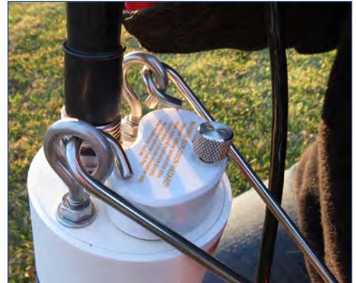
7. Attach serial port end to the Surveyor.
