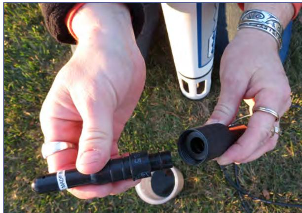
5. Line up the raised dot on the cable with the large prong. Be careful with the pins!
