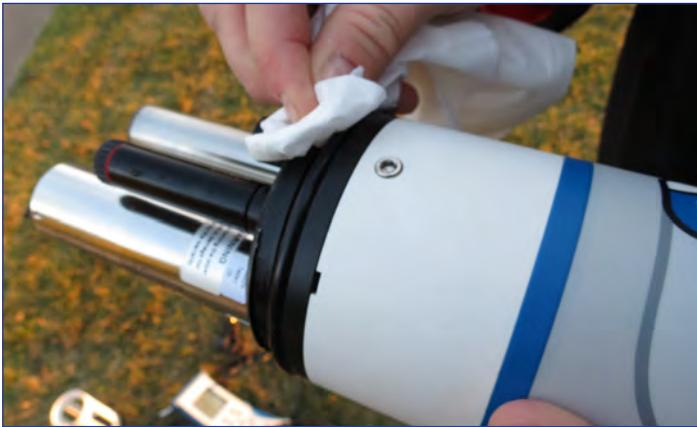
10. Attach calibration cup to the Hydrolab. Screw on and then back off  $\frac{1}{4}$  turn. Allow at least 5 minutes for the air to become saturated with water.
